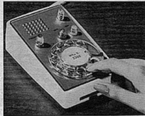
▼ A compact microphone-dial unit for "hands-free" telephoning.
