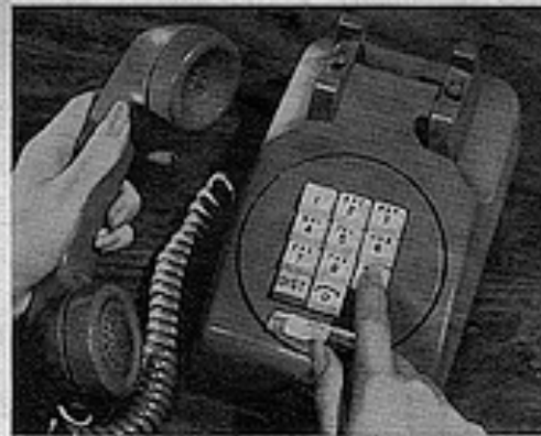
▲ A phone that has push buttons instead of a dial for calling.
